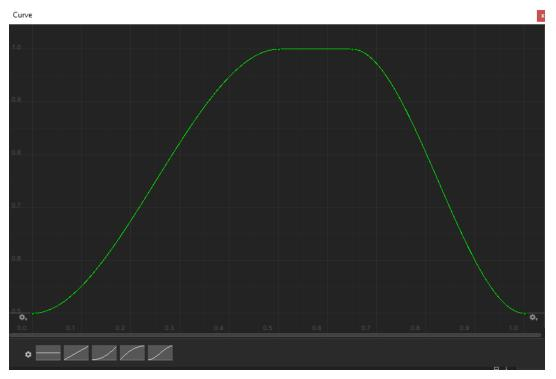
The curve represents the percentage of the peak temperature over time of day. The default lowest value is set to 0.5 (i.e. 50%) at time 0. Therefore, you will get 50% of the peak temperature at midnight. Near the center of the graph the default is set to 1.0 (i.e. 100%). After a few hours, the curve drops down again towards 0.5 at the end of the day cycle. You can modify this curve any way you want to get the desired range of temperatures throughout the day.
